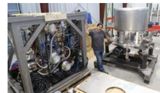
SHINE founder Greg Piefer with one of SHINE's neutron generator systems
